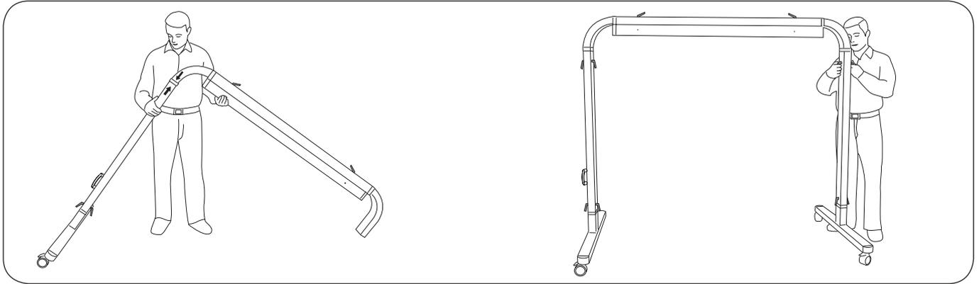
1. Fit the rail to one of the side supports, as in the illustration. Make sure the handle is facing outward. Mount the upper locking handle that holds the rail to the side support, and tighten.
