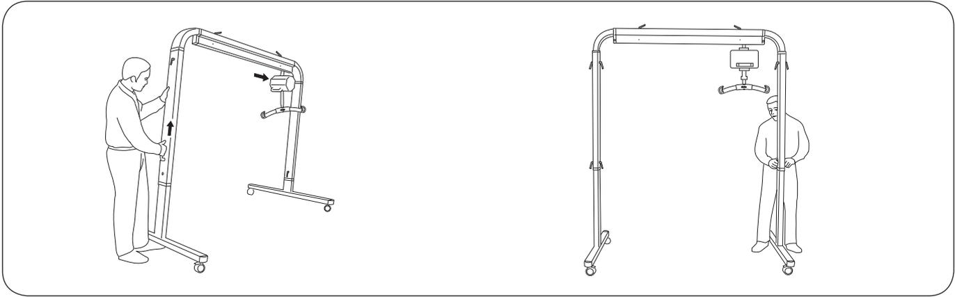
5. Now FreeSpan is ready to be raised to the correct height. There are four different height positions.
