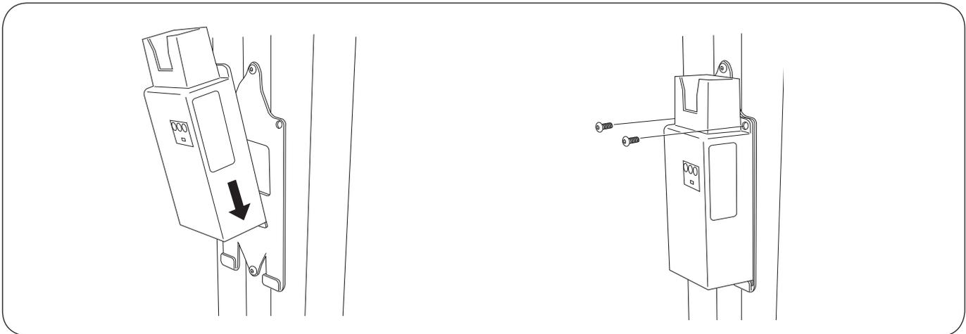
Hook on the lower part of the charger on the pre-mounted charger plate (as illustrated).
