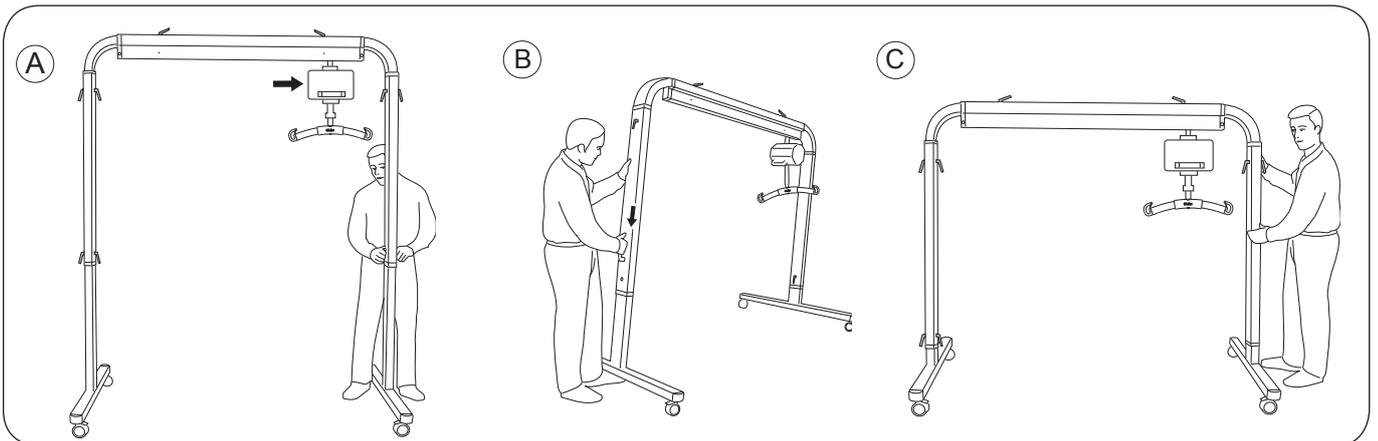
A) Start by moving the lift unit to the side that is to be lowered first. Loosen the locking handle, remove it and lower the side support to the lowest position. Hold the handle firmly to maintain a secure grip.
