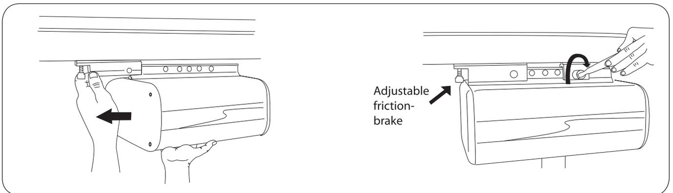
Unscrew the bolt and nut that is mounted in the carriage. Slide the lift unit onto the longer carriage with the emergency stop end in the opposite direction as the carriage brake knob, as in the illustration above. Affix the carriage in the outermost hole in the mounting rail above the lift unit using the accompanying bolt and nut.
