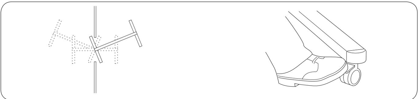
**Helpful hint.** Where door openings are narrower than 1240 mm (48.9 in.), move the lift according to the illustration above (zigzag).
