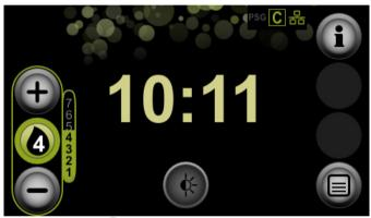
The and buttons can be used to increase or decrease the humidifier level.
