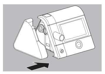
7. To use the therapy device without the respiratory air humidifier in the future, insert the cover in the therapy device from the side until the unlocking button clicks into place audibly.
