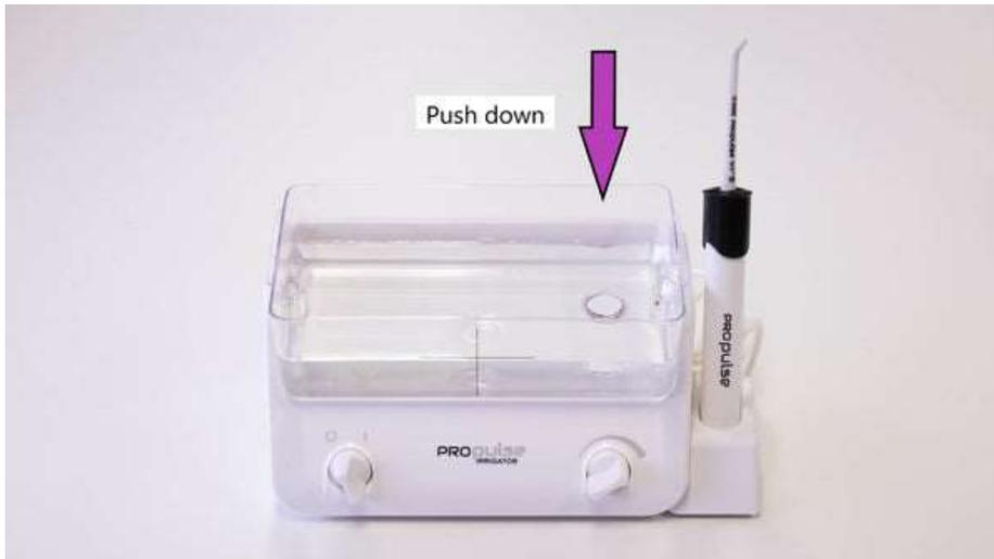
If your unit is still not producing the correct water flow, check the plug hole on the upper casing of the ProPulse®, the handle and the QrX™ tip for any potential blockages.
