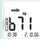
The meter will store the data of one code strip per test parameter.
