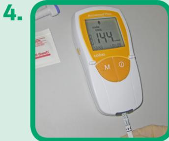
If your test/code is not displayed it will be necessary to insert the code strip for the test strip lot you wish to use.
