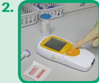
Place the instrument on a level, vibration-free surface and switch on by pressing the On/Off button.
