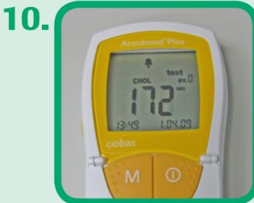
Close the chamber flap. This starts the measurement & countdown.
