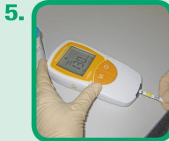
Remove a test strip from the container and close the container immediately. Check its appearance for discolouration. Do not use if discoloured.
