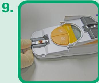
Insert the test strip back into the instrument.
