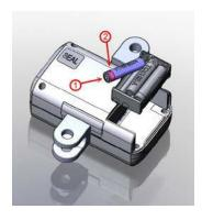
4.Installing 6\* AAA size batteries.
