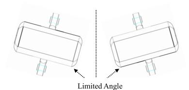
Cardon joints are assembled with loadcell from ex-factory. It should not be twisted by user or in any other circumstance. Misusage will cause unexpected danger.
