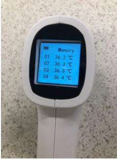
From the off state press and hold trigger button to view first 4 readings
