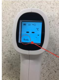
Ensure the screen shows that the unit is in Body mode
