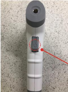
Press the “on” button once quickly and release pressure off the trigger
