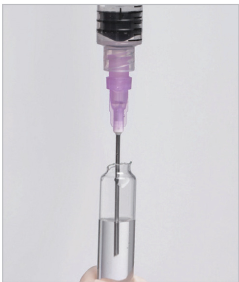
5-micron filter needle for use with glass ampules. Prevents glass particles from entering the syringe.
