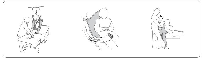
Position the patient above the bed. Raise the head end of the bed for the patient's comfort. Lower the patient onto the bed. Remove the leg supports by pulling out the leg support loops under the fabric part of the leg support. **Tip:** This is facilitated if the patient's legs are bent. Remove the sling by carefully pulling it up.
