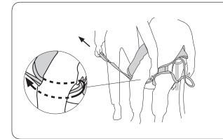
Carefully remove the leg support. The gentlest way of doing this is by pulling out the leg support loops under the fabric part of the leg support.
