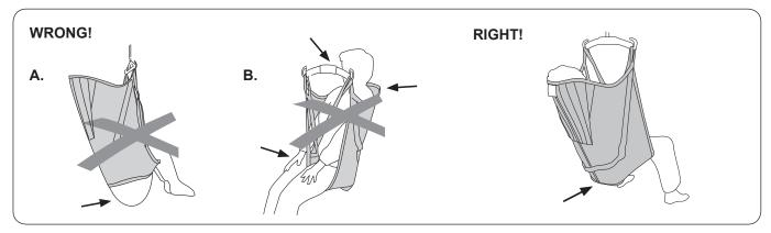
**A. Risk of sliding out.** The buttocks hang down. The sling may be too large. It can also be due to the fact that the sling has not been pulled down the patient's back sufficiently.
