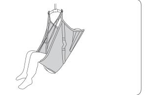
**Tip:** Check that all suspension loops have the same length, i.e., are at an equal height when they are stretched prior to lifting. Adjust the position of the sling if they are not at an equal height.
