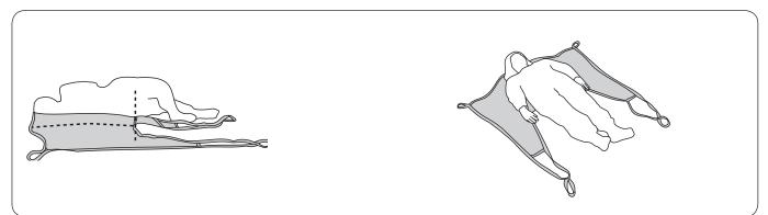
Carefully turn the patient onto the side and place the sling's edge under the patient with the lower edge **level with the coccyx.** Fold the sling so that its centre back strap corresponds to the patient's spine when the patient is turned back again gently. Carefully pull the sling out from the other side.
