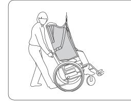
When placing a patient in a wheelchair: Lean the chair backwards during the lowering of the patient. Let the buttocks slide down the backrest during the last part. Control the angle of the wheelchair with your foot on the tipping support.
