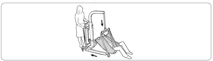
When lifting to the floor, the wheels of the lift should not be locked. When the patient touches the floor, the lift should be pulled backwards to give space for the head. **Tip:** If lifting is to a thinner gym mat, the lift can be pushed in under this mat, so that the mat acts as a soft protection between the lift and the patient. If the sling is to be removed, see "Removing the Sling when the Patient is Lying in Bed", page 6.
