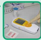
Place the instrument on a level, vibration-free surface and switch on by pressing the On/Off button.
